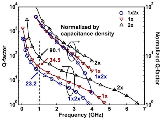
Fig. 4. VPP capacitor *Q*-factor plots. *Q*-factors are estimated from pre-de-embedding data due to singularity in the de-embedded *Q*-factor. The 1x, 2x, and 1x + 2x capacitors show *Q*-factors of greater than 34.5, 90.1, and 23.2, respectively, at 1 GHz. In the normalized *Q*-factor per unit capacitance plot, the 1x + 2x capacitor's *Q*-factor scaling effect by capacitance is observed. The normalized plots are shifted upward for visualization.
