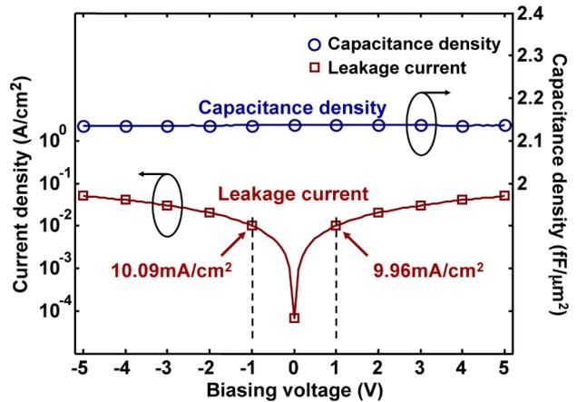
Fig. 6. Leakage current and capacitance densities with dc voltage biasing to the 1x + 2x VPP capacitor. The capacitor shows symmetric leakage current, and a current density of about 10<sup>-2</sup> A/cm<sup>2</sup> is observed at ±1 V. The capacitance density is 2.13 fF/μm<sup>2</sup> at 200 MHz, and its voltage linearity is less than 80 ppm/V<sup>2</sup>.
