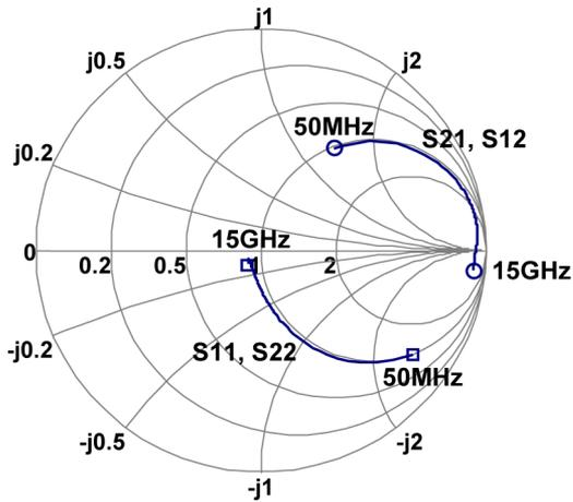
Fig. 2. VPP capacitors' *S*-parameter measurements Smith chart plots from 50 MHz to 15 GHz. The S21 and S12 plots are mapped on the same trace; so do the S11 and S22 parameters.
