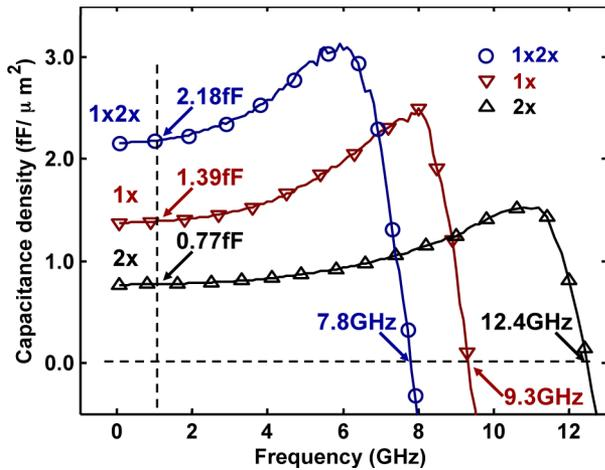
Fig. 3. Density plots of the 1x, 2x, and 1x + 2x VPP capacitances. The capacitors show capacitance densities of 1.39, 0.77, and 2.18 fF/μm<sup>2</sup>, respectively, at 1 GHz. Each VPP is 100 μm by 100 μm. The 1x + 2x capacitance is the sum of the 1x and 2x capacitances within 1% error.
