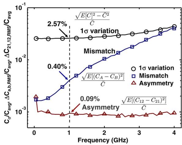
Fig. 5. Statistical characteristics of the 1x + 2x VPP capacitor. The 1σ variation is 2.57%, the rms mismatch is 0.40%, and the rms asymmetry is 0.09% at 1 GHz. The rms capacitor asymmetry is about 60 dB below the capacitance value.
