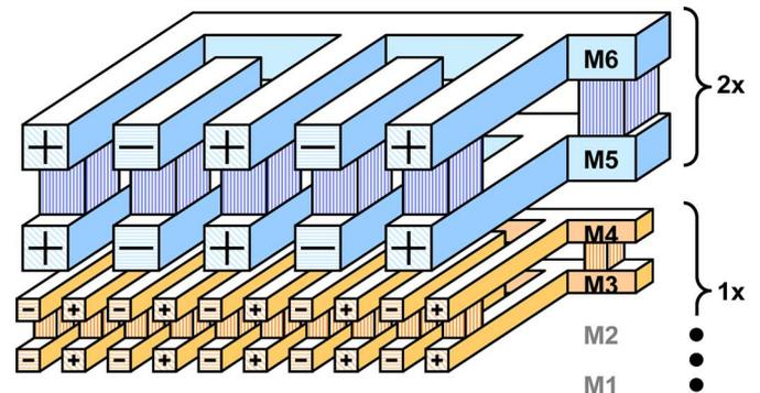
Fig. 1. VPP capacitor layout diagram. The upper two layers of the  $1x$  layer (M3 and M4) and the  $2x$  layers (M5 and M6) are shown. Interdigitated metal lines and interlayer vias are placed to maximize capacitance density and manufacturability.
