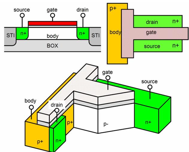
Fig. 1. SOI floating-body and body-contacted FET diagrams. The buried oxide layer effectively reduces diffusion volume and parasitic capacitances. A body contacted device is formed with a T-shaped gate and PN junction for analog design. Partially-depleted FETs are implemented in 65nm SOI CMOS.
