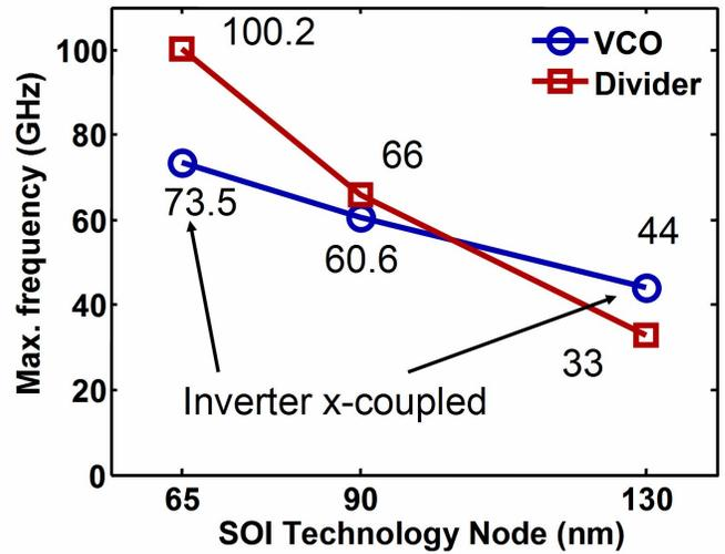
Fig. 6. SOI CMOS based LC-VCO and CML static divider performance scaling. The VCOs in 65nm and 130nm used complementary topology that employs both NFET and PFET negative  $g_m$  pairs. Considering PFET's lower DC and RF performances, the scaling has been effective in both FETs. The divider scaling has been stronger, and the VCO oscillation frequency is more affected by LC-tank and wiring parasitics.
