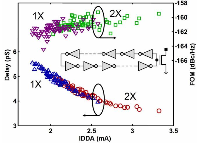
Fig. 3. Inverter-based 101-stage ring oscillator stage delay and phase noise measurements on a 300mm development wafer. The minimum gate delay record is 3.6psec. The 2X pitch RO is faster than 1X by 16.9%. The phase noise figures-of-merit are almost same in both ROs.
